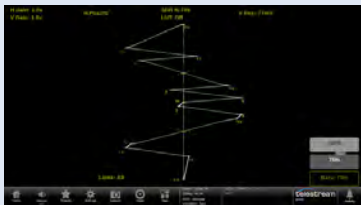
Using a simple color bar test pattern 75% or 100% should align within the appropriate graticule boxes.
