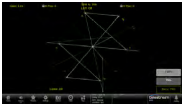
Selectable Bar Format for 75% and 100% Graticules with input selection for chromaticity of 709 or 2020.
