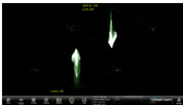
Split Diamond display that allows the user to see the offset in the black of the RGB color components.
