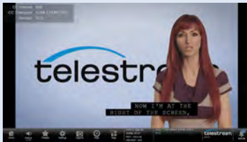
Closed Captions or subtitles can be decoded and displayed in CEA 608/708 or OP47/ST2031 with the ENG-QC option.
