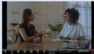
Lightmeter provides relative exposure values in Stops or Nits with up to five cursors that can be position within the image available with option PROD.
